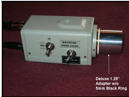
Remove plastic lens cap and 5mm black extension ring. Install deluxe 1.25" aluminum adapter. If a MFR-3 focal reducer is to be used, either place the 5mm black or the 10mm aluminum extension ring between it and the camera.
