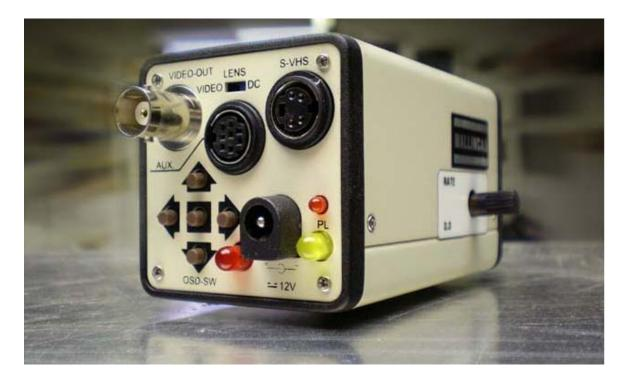
This is the opposite end for all the connections. The brown buttons are for manual on-screen menu control. The center plug-in is for an optional remote serial camera control. If you are using a computer in the field, there is a software application (covered later) that can control the camera, (a serial to USB converter will have to be purchased if you are using a newer computer).
