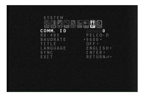
COMM. ID, RS-485 and BAUDRATE will come into play once the software has been developed and the communication cable prepared. For now, leave the COMM ID to 1 and the BAUDRATE to 9600.
