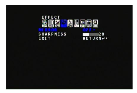
The MIRROR function can either be OFF, which leaves the image on the monitor unaffected or it can be set to HOR, VERT, or ROTATE. These last three MIRROR options allow alteration to how the image appears on the monitor.
