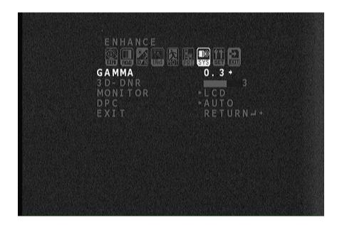
There are four GAMMA settings -0.3, 0.45, 0.6 and 1.0. GAMMA 0.3 will provide the brightest image on the monitor and GAMMA 1.0 will provide the darkest image. Select the GAMMA value that provides the most pleasing image on the monitor.
