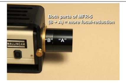
Here's the complete MFR-5 screwed together and mounted on the camera
