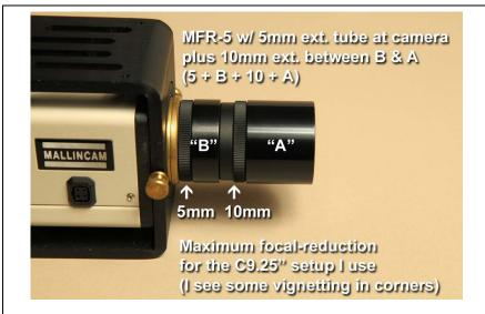
And you can combine extension tubes between part "A" and part "B" at the same time as adding an extension tube between the camera and the back of the MFR-5. This can result in a LOT of focal-reduction – even too much!
