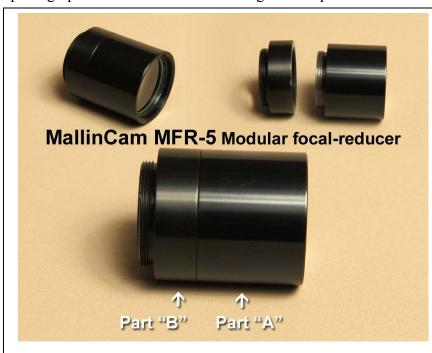
Here are three images of a MFR-5 focal-reducer. It's a two-piece design and is made to mount on C-mt. video cameras, is 1.25" in diameter and has 1.25" filter threads on the end of the larger part I call the "A" part.
