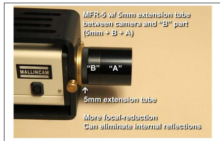
You can also put extension tubes between the camera and the MFR-5. This also increases the amount of focal-reduction.
