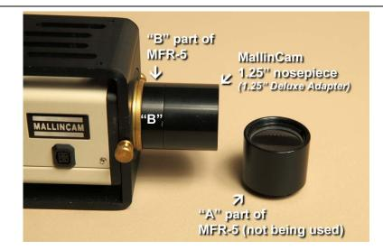
And here it is with a MallinCam 1.25" Deluxe adapter (nosepiece) screwed into the open end of the "B" part. This is the 1.25" nosepiece that came with my MallinCam Xtreme camera – you don't need to buy another one.
