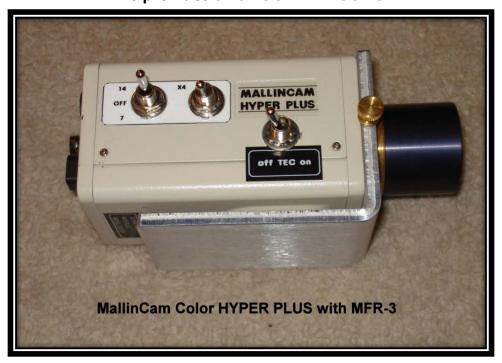
They look the same. The only way to tell them apart is to look into the front of the machined aluminum barrel to see if there is a lens present. Adding a 10MM Extension Ring between the MallinCam and the MFR-3 provides a 0.65 FOCAL REDUCTION.
