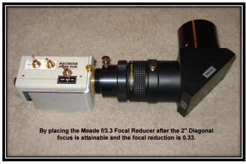
If the ScopeStuff 2" Female Barrell to Female Schmidt Thread Adapter with Compression Ring is removed, then the assembly can be placed into a 2" focuser on a refractor for wide field viewing
