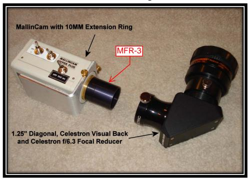
The assembly is screwed directly to the back of the SCT Optical Tube Assembly and the system speed will be f/4.
