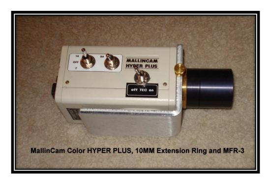
If additional focal reduction is needed, a second 10MM Extension Ring can be inserted between the MallinCam and the first 10MM Extension Ring.
