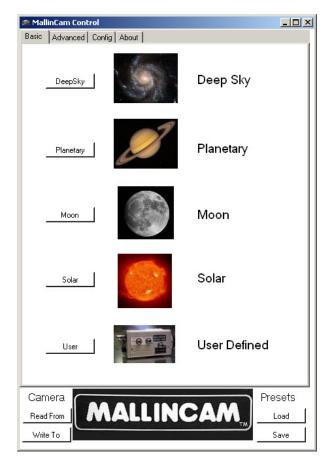
This screen contains five pre-programmed buttons for easily changing between DeepSky, Planetary, Moon, Solar, and User Defined modes. Whenever one of these buttons is depressed, the "Camera" label next to the "MALLINCAM" name at the bottom of the window will change to "Sending" and be highlighted in RED
