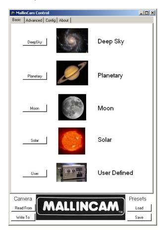
Start the control software, and if everything is properly configured, the MallinCam Control "Basic" Window will appear on your computer screen. However, the control software defaults to COM1, and your Serial device may actually be on a different Port. If so, the following ERROR Message will be seen when the control program is first started.
