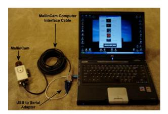
The above figure shows how the MallinCam is connected to the computer using the Control Cable. If your computer does not
