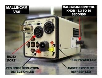
MallinCams with a GREEN power LED have an RS485 computer interface. MallinCams with a RED power LED possess an RS232 computer interface. If your MallinCam possesses either interface, a computer can control it. Proceed to STEP TWO
