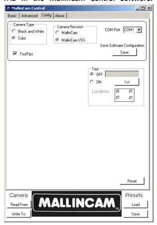
The window seen above will appear. Go to COM Port and select the one that your Serial device is on (COM1 through COM9). Also select the Camera Type (Black and White or Color) and the Camera Revision (MallinCam or MallinCam VSS). Then click the "Save" box and exit the program entirely. Restart MallinCam Control Software and it should open the "Basic" window shown below.
